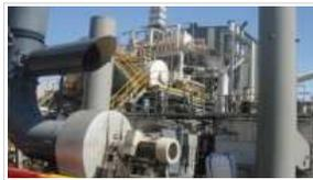
Power plant uses coal mine ventilation air as fuel
